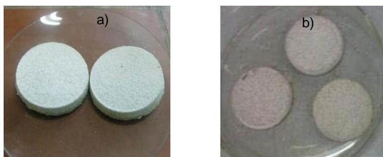
**Fig. 1 Membranas:(a) Vítreas (b) Zeolita natural cubana.**
