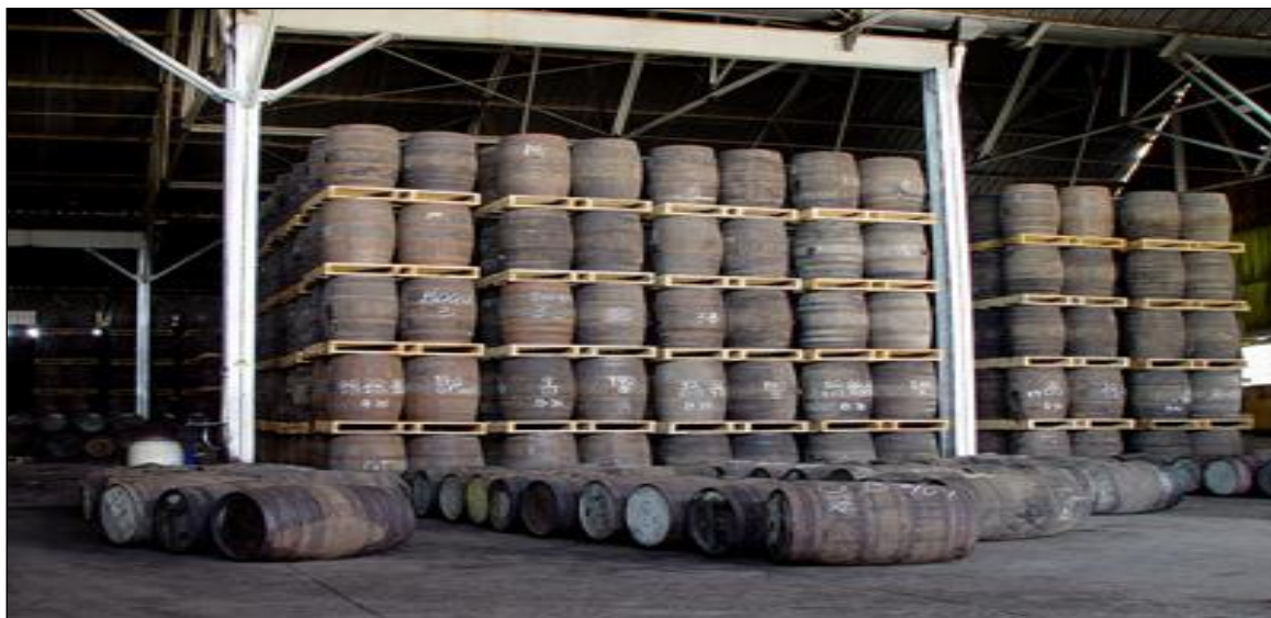
Fig.1- Palletized ageing system. Barrels are stored in vertical position. (picture with the permission of the major rum producer of Cuba)
